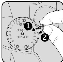
Flexion and extension positions can be restricted to 0°, 15°, 30°, 45°, 60°, 75° and 90°. The wedges are pushed into the lateral interlocking and locked downwards by being lodged. The A/B labelling of the wedges here is in your direction. Ensure that the angled wedge is set at the desired number of degrees.
