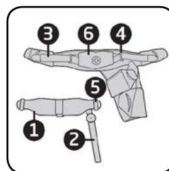
**1 / 2** Remove the pelvis buckle including the joint by detaching the lower articulated shank ② from the Velcro fastener area. Then, thread the narrow straps ③ which are guided around the pelvis buckle out of the guide loops ④ and passage loops ⑤ of the pelvis buckle.
