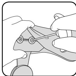
Detach the screw-type connection which joins the brace joint to the pelvis buckle. This connection is located under the cover on the inside of the pelvis buckle in the region of the joint.
