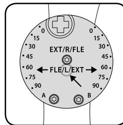
When adapting for the RIGHT-HAND side of the hip, the restriction for flexion can be found under the marking "FLE" on the right-hand side and the restriction for extension under the marking "EXT" on the left-hand side of the joint.
